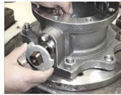
Figure 13 - Installing Stop Plate
