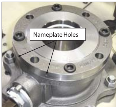
Figure 21 - Name Plate Holes Orientation
