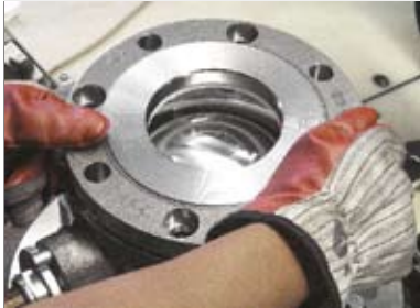
Figure 20 - Placing Cap Plate on Body
