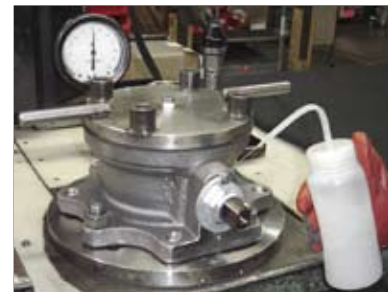
Figure 14 - Valve Stem Leak Test
