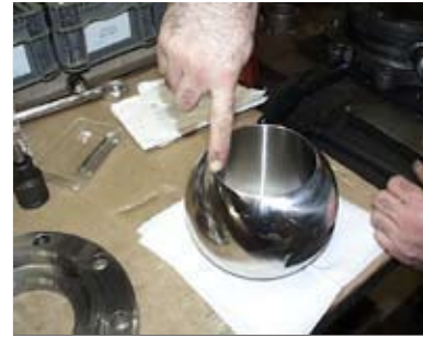
Figure 17 - Checking for Nicks
