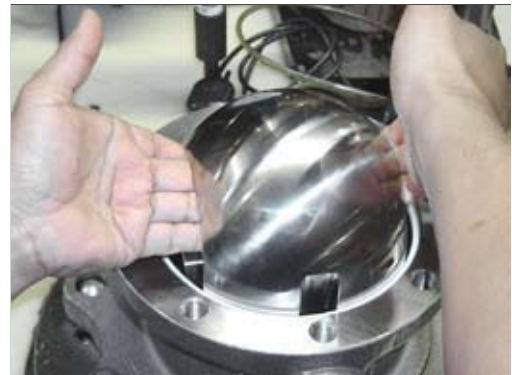
Figure 6 - Valve Ball Removal
