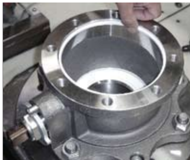
Figure 16 - Body Seal Installation
