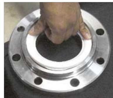
Figure 19 - Installing Ball Seal in Cap Plate
