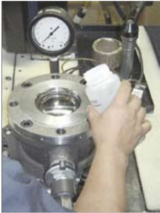
Figure 25 - Immersing Seal for Leak Test
