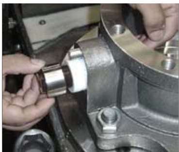
Figure 12 - Installing Packing and Spacer
