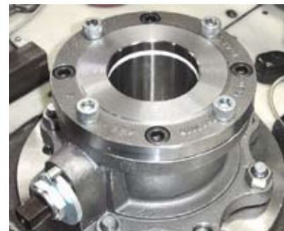
Figure 3 - Ball Valve in Open Position
