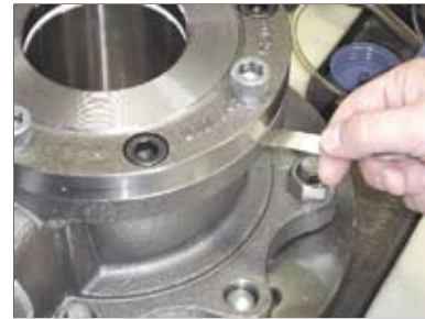
Figure 23 - Checking Cap-to-Body Contact
