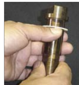
Figure 10 - Installing Thrust Washer
